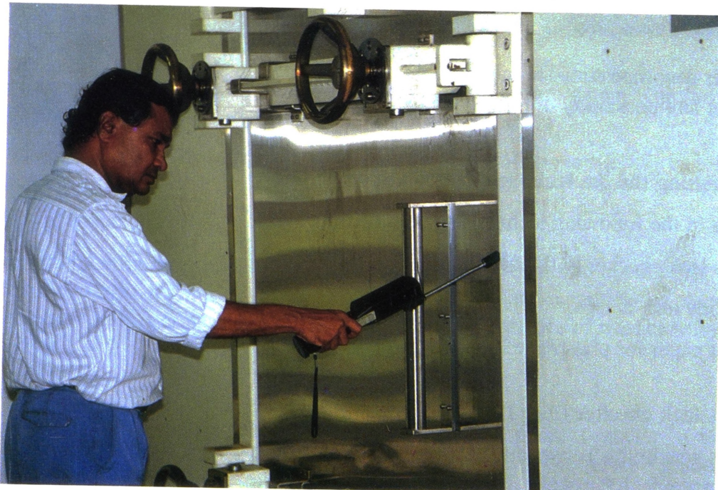
Fig. 10 Checking the door beading with the gas leak checker for methyl bromide gas leaks
