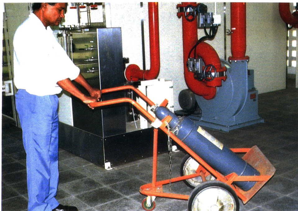
Fig. 5 Transportation of compressed liquid methyl bromide steel cylinder fixing on a cart
