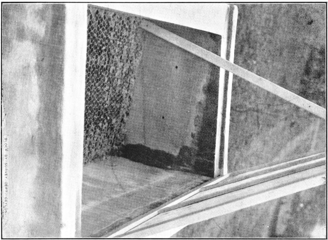
Fig. 8. Closer view of the propagating chamber showing the wire netting resting on expanded metal. Below this extends the heating chamber containing water
